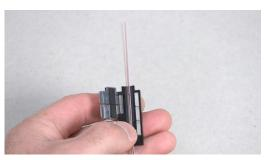
2. Load the ribbon into the holder. Start with approximately 40mm of the fiber extending from the end of the holder.
