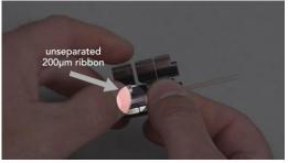
4. While holding the ribbon in place with a finger, close the first hinge lid to hold the unseparated 200um portion of the ribbon.
