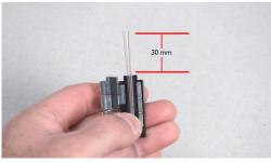
3. Anchor the fiber with your thumb and pull fiber back until there is 30mm of fiber extending from the end of the holder.
