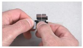
5. Slide a finger on the fibers from the closed first lid to the end in order to push the fibers into the V-grooves. Hold the fibers in the V-grooves with a finger and close the second lid.
