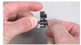
6. Pull the ribbon a little at the end to ensure that each fiber is set in order on each v-groove, then close the third lid. Complete.
