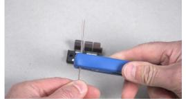
1. Split the 200um rollable ribbon into single fibers at the end by running the ribbon through the RST-01 three times.
