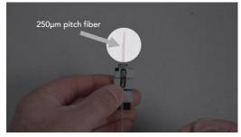
7. After the pitch conversion process is complete, strip, clean, dry and cleave the ribbon fiber before loading into the fusion splicer.
