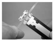
2) Confirming that S233 doesn't pinch the ribbon, with moving slightly. If S233 doesn't move well (nothing the sticking), do procedure 1) again.
